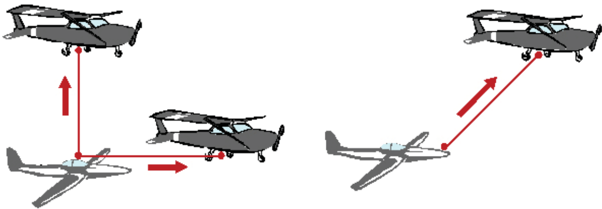
Figure 1: The vertical and horizontal forces required to pull a glider into flight can be achieved with one tow rope.
